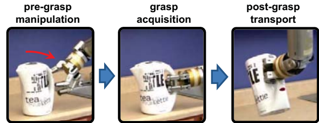
Fig. 1. A fetching task requires a complete manipulation plan including grasp acquisition and transport. We present a method for incorporating pre-grasp manipulation, specifically object rotation, in the manipulation plan. The object adjustment resulting from pre-grasp manipulation increases the task success rate and improves the quality of the transport plan.
