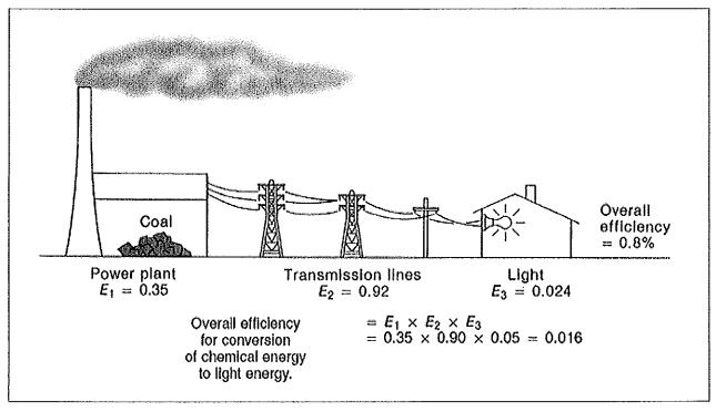
FIGURE 2 Lighting efficiency. Source: NRC, 2009.
