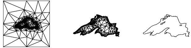
Figure 1: Incremental mesh refinement algorithms first generate a mesh over a bounding box (left), then remove the scaffold vertices and elements (center). Some applications are interested in only the surface mesh (right). The one-dimensional Lake Superior surface mesh shown has 530 surface vertices. The volume mesh shown has 1072 total volume vertices; 258 interior and 284 exterior. We offer the first theoretical analysis of the costs of this scaffolding.
