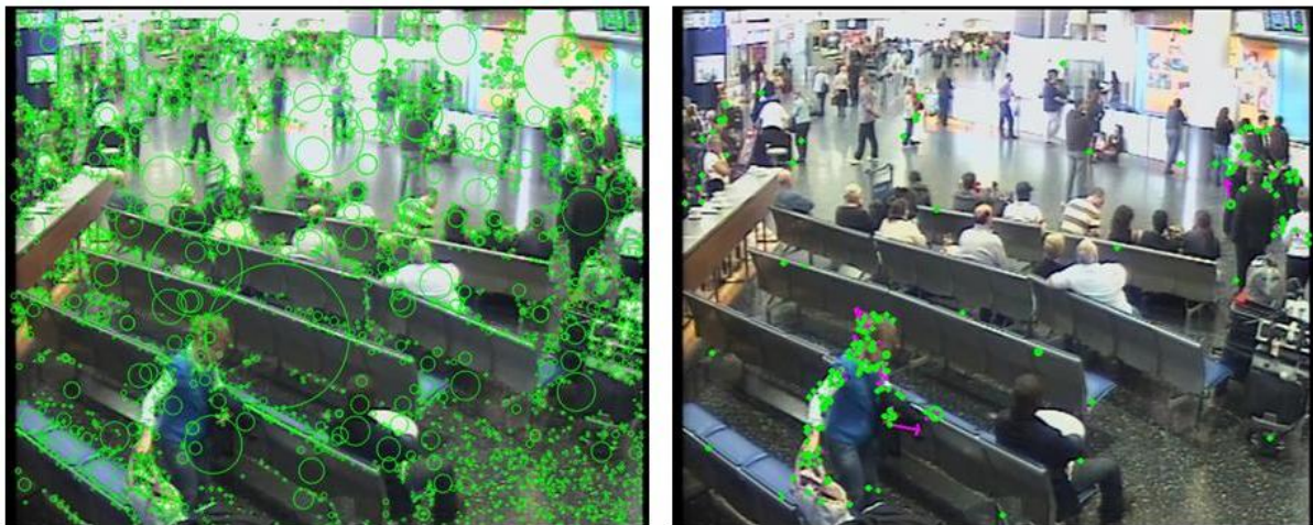
Figure 6: Interest points detected with SIFT (left) and MoSIFT (right). Green circles denote interest points at different scales while magenta arrows illustrate optical flow. Note that MoSIFT identifies distinctive regions that exhibit significant motion, which corresponds well to human activity while SIFT fires strongly on the cluttered background.
