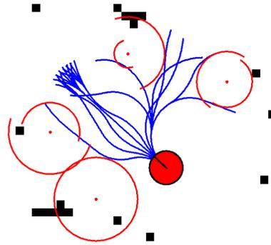
A heuristic function selects goal-directed local paths from a set of 2,401 paths. A low-fidelity global planner helps guide the robot to the goal. In order to assess the effect of various path sampling strategies, we varied replan cycle time. Fig. 10 shows a screen capture of our simulator, indicating known collision sites (in C-space) and ranges of effect. We consider four path sampling strategies:
