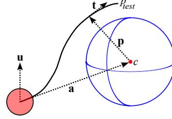
possible approach is to shrink the range of effect for the obstacle at  $c$ , as in Fig 6b, which supposes that the obstacle is smaller than initially thought. Another approach, to shift the entire distribution away from the safe path as in Fig. 6c, assumes that the obstacle size was correctly estimated, but its position was off.
