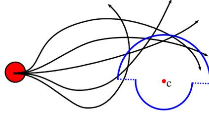
to the collision point,  $c$ . This assignment of paths to a single side of an obstacle places assumptions on the path's shape. We assume here that curvature is bounded and that paths are reasonably short. Previous work by Knepper, et al. [15] thoroughly discusses these assumptions.
