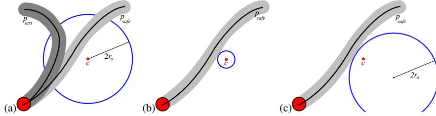
**Fig. 6** (a) Given a collision point  $c$  and neighboring collision-free path  $p_{safe}$ , the blue circle represents a distribution on obstacle locations, some of which are invalidated by  $p_{safe}$ . The more distant candidate path  $p_{test}$  is not at risk of collision with the obstacle represented by  $c$ . (b) and (c) Two simple hypotheses on obstacle scale and position explain these two results. The distribution shown in Fig. 4(b) is simpler to represent during online path sampling.
