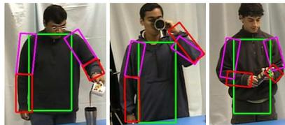
Figure 6. Results of Upper Body Pose Estimation Algorithm.
