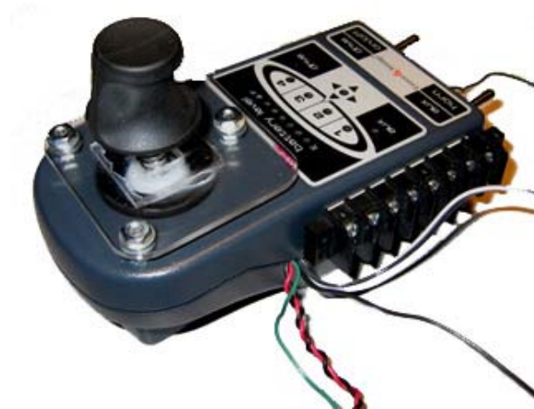
Figure 6: The Everest & Jennings 1706-5020 power wheelchair joystick we modified for EdgeWrite text entry. Note the plastic template around the stick, which provides a square boundary.
