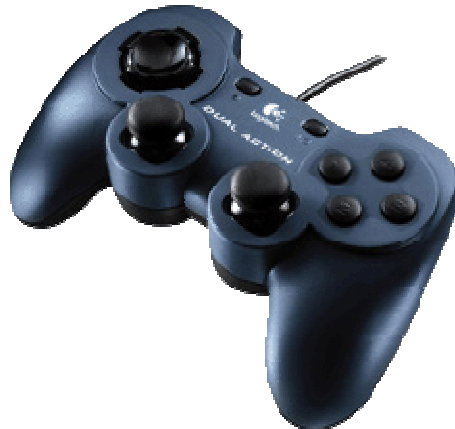
Figure 5: A game joystick showing the two thumbsticks which can be used to enter EdgeWrite. Each thumbstick is set within a square area.
