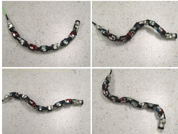
Fig. 1: Examples of a snake robot executing the gaits discussed in this paper. Moving across from top left to bottom right: rolling, sidewinding, slithering, and turn-in-place.
