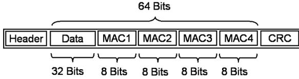
**Figure 1. Example packet containing 32 bits of data and four 8-bit MACs, for four receivers.**
