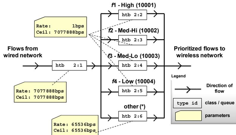
Figure 2: HTB Qdisc Configuration
