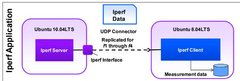
Figure 6: Iperf Application Configuration
