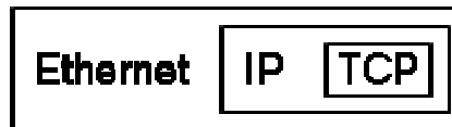
a TCP packet embedded inside an IP packet, embedded in an Ethernet frame
