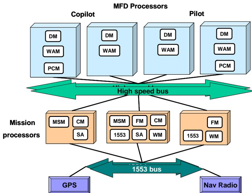
Figure 2: Typical Documentation of Avionics System Architecture
