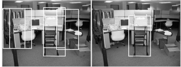
Figure 5. Left: Example of scanning an edge density filter for the ladder over a raw edge image (left) and an edge image which has been filtered using the technique described in Section 2 (right). See section 3.3 for details.
