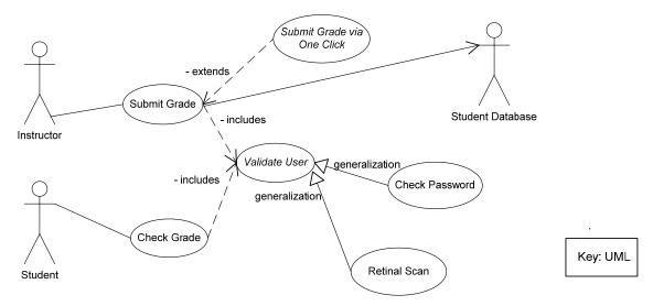
Figure 1: Partial Use Case Diagram for Online Course Management System
