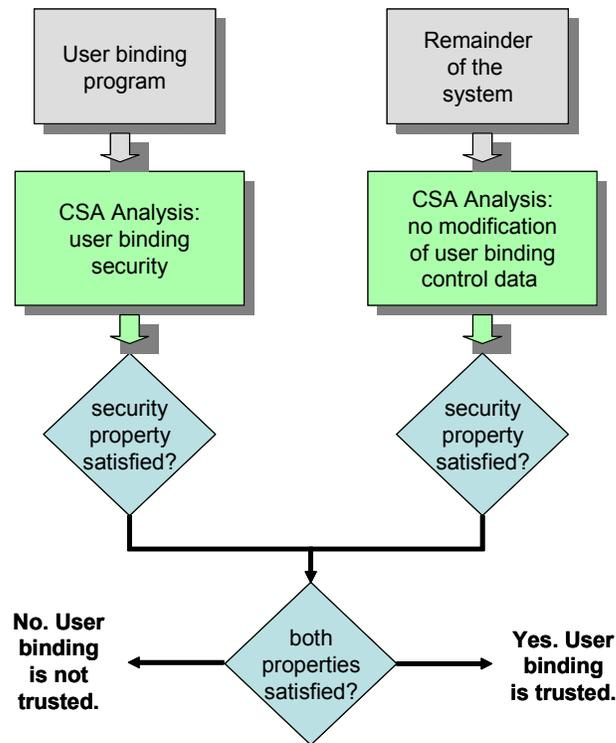
Figure 11: CSA Analysis of Trusted User Binding
