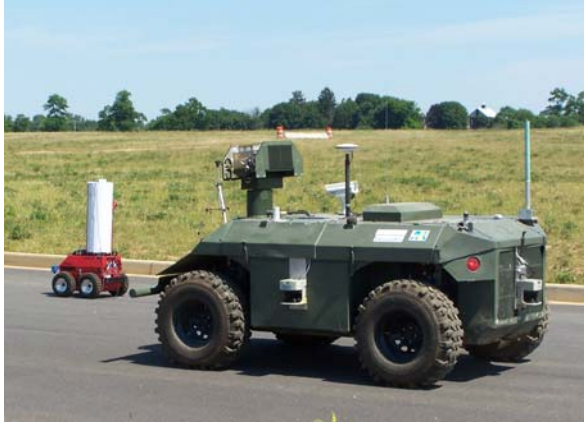
Figure 1. A Demo III Experimental Unmanned Vehicle (named XUV), and a smaller robot used as a controlled target for establishing ground truth.
