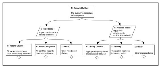
Figure 6: A Possible Top-Level Safety Case Structure
