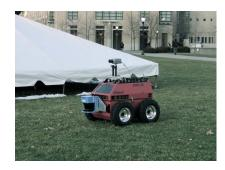
Fig. 5. Our experimental plaform is based on an ATRV-JR equiped with a firewire camera and SICK laser range finder. The vehicle planner [16] and laser processing run on the robot. The image processing is done off-line and results are send back to the robot.
