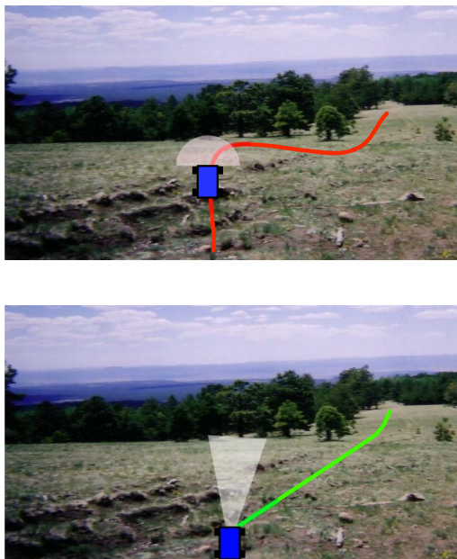
Fig. 1. Top: poor performance due to lack of sensor planning and mid-range sensing, the robot has to rely on mobility sensor data only. Bottom: the pinch point is detected earlier, which allows the planner to adjust the path accordingly.
