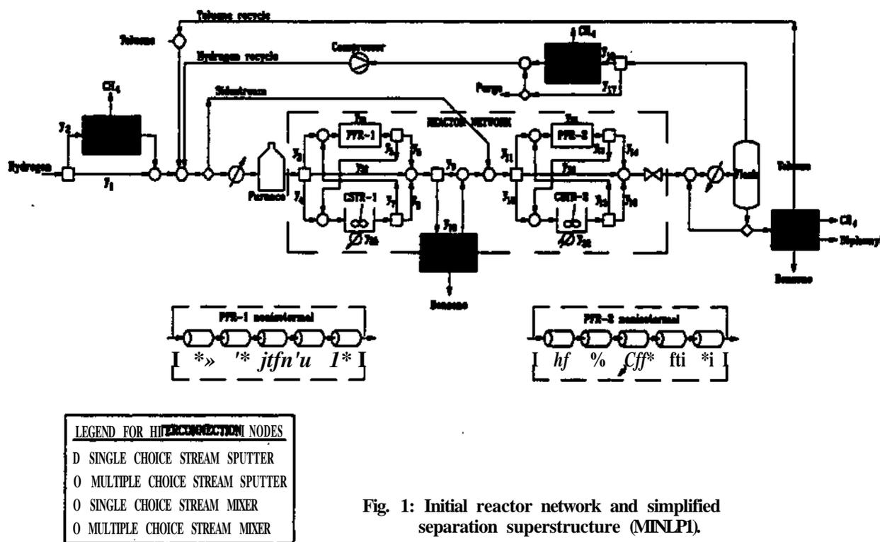
Fig. 1: Initial reactor network and simplified separation superstructure (MINLP1).
