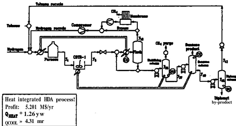
Fig. 6: Optimal flowsheet and its heat integrated HEN (MINLP3).
