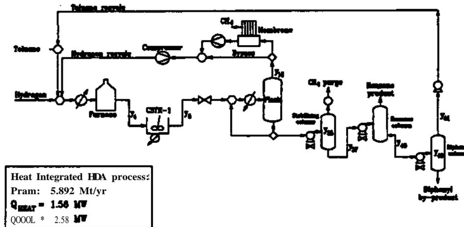
Fig. 4: Optimal flowsheet of expanded superstructure without HEN (MINLP2).
