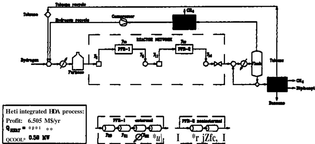
Fig. 2: Optimal structure for initial superstructure problem (MINLP1).
