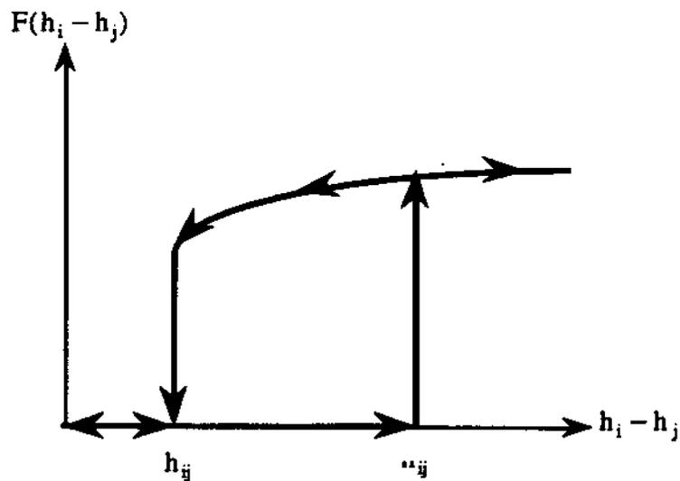
Figure 4: Hysteresis curve showing flow in the pipes
