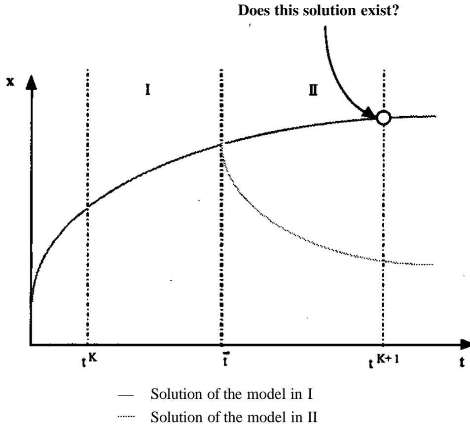
Figure 2: Existence of solution in discontinuity locking methods
