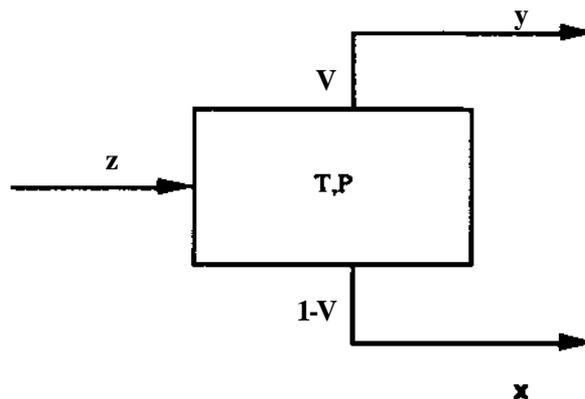
Figure 8: Isothermal flash operation
