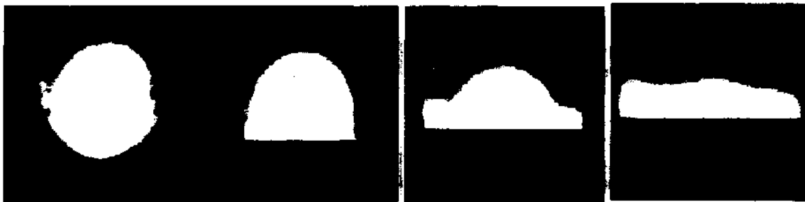
Figure 6, High Speed Photography of Stainless Steel Droplet Spreading (Images at time of impact, and 0.001, 0.002 and 0.003 seconds after impact).
