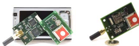
Figure 1. Split- and single-board sensor board designs.
