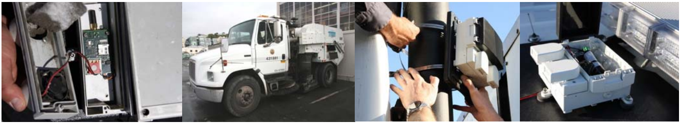
Figure 2. Variants of the sensing platform, enclosure-mounted on city street sweeping vehicles.
