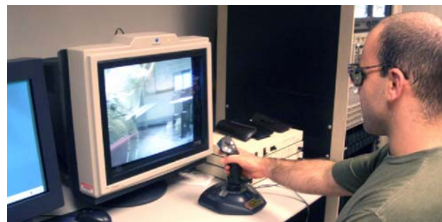
Figure 4. Initial workstation with stereoscopic telepresence capability.
