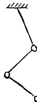
Figure 5. A multiple pendulum.
