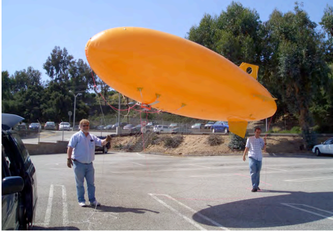
Figure 13. The TAOSF aerostat observation platform. The photo on the left shows the aerostat, which is an unmanned, lighter-than-air (LTA) unpowered blimp on a tether. Helium is used for buoyancy. The gimbaled TAOSF observation platform avionics package is shown on the right. It includes a GPS, a barometric altimeter, a magnetic compass, a serial wireless data link, a wide-angle color camera, and a video transmitter.
