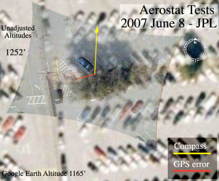
Figure 14. Initial results from the TAOSF aerostat observation platform. Tests of the ground truthing system were conducted. By registering aerial imagery to satellite imagery, the overall uncertainty in the ground position estimates derived from the aerostat platform were estimated. The camera image (in grey) was taken when the aerostat was 30 m above ground.
