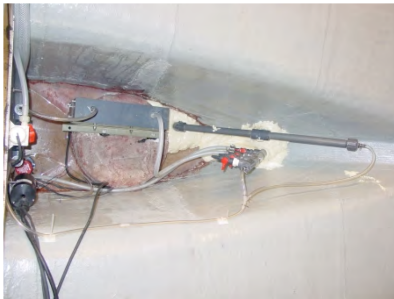
Figure 5. OASIS forward payload bay with salinity and chlorophyll sensors installed.
