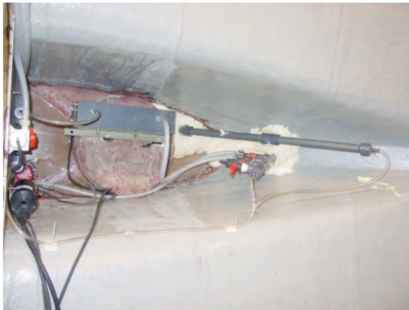
Figure 5. OASIS forward payload bay with salinity and chlorophyll sensors installed.
