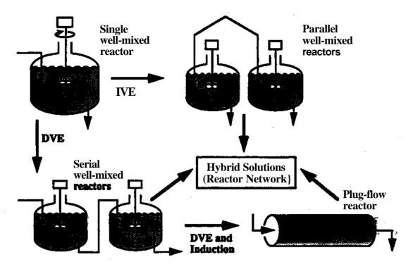
**Figure 3.** Application of 1<sup>st</sup>PRINCE to chemical reactor design
