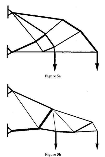
**Figure 5:** Truss structures generated by shape annealing topology without buckling constraints (5a) and with buckling constraints (Sb) (from Reddy and Cagan, 1993)
