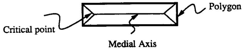
Figure 2: Example of MAT for a simple polygon
