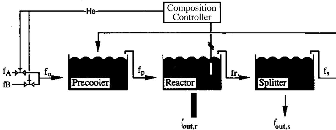
Figure 3-2. Introduction of a Composition Controller
