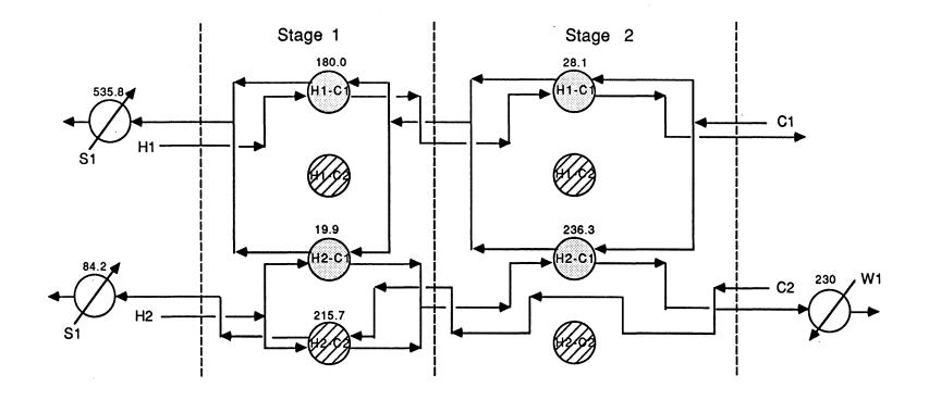
Figure 4 Example 1 Feasible Network Achieving Area Target
