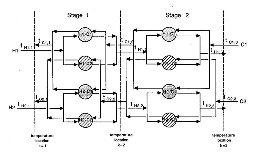
Figure 2 Two Stage Superstructure
