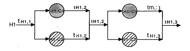
Figure 3 Restrictions on Split Temperatures
