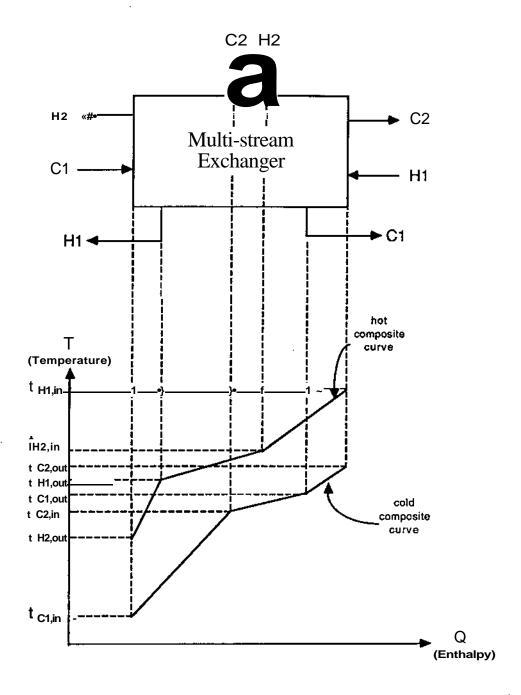
Figure 6 Representation of Multi-stream Exchanger on Composite Curves
