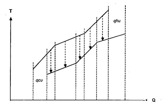
Figure 1 Vertical Heat Transfer Between Composite Curves
