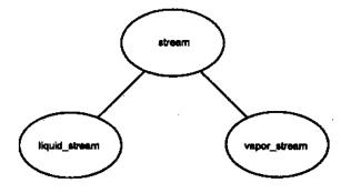
Figure 2. An Inheritance hierarchy for describing material streams.
