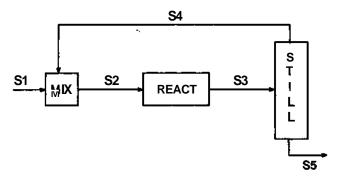
Figure 1. A simple flowsheet with a recycle stream.
