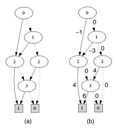
**Fig. 2.** (a) Reduced BDD for  $2x_0 + 3x_1 + 5x_2 + 5x_3 \ge 7$  using the variable ordering  $x_0, x_1, x_2, x_3$ . (b) Same BDD with edge lengths corresponding to the objective function  $2x_0 - 3x_1 + 4x_2 + 6x_3$
