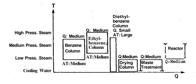
Fig. 3 Qualitative Assessment of Heat Loads -fat-Liquid Phase Reaction Alternative
