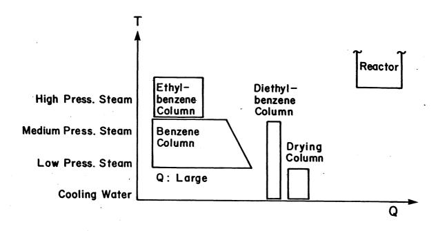
Fig. 4 Qualitative Assessment of Heat Loads for Vapor Phase Reation Alternative
