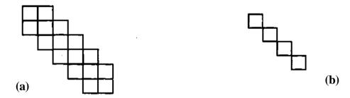
Figure 6: End view of a plate at 45 degrees to the axis, and it's skeleton
