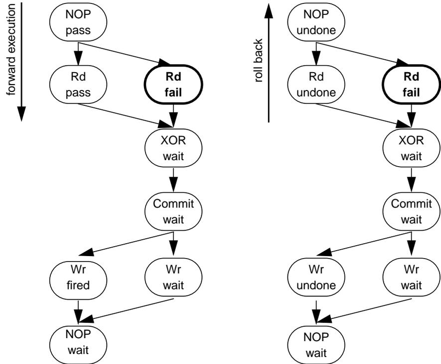
The failure of the Rd node (indicated in bold) occurs prior to the commit point. This causes forward execution to halt and roll back to begin. Roll back works backward through the graph from the point of failure, undoing the previously completed nodes. If a failure occurs prior to the commit point, the system appears as if the graph never executed.
