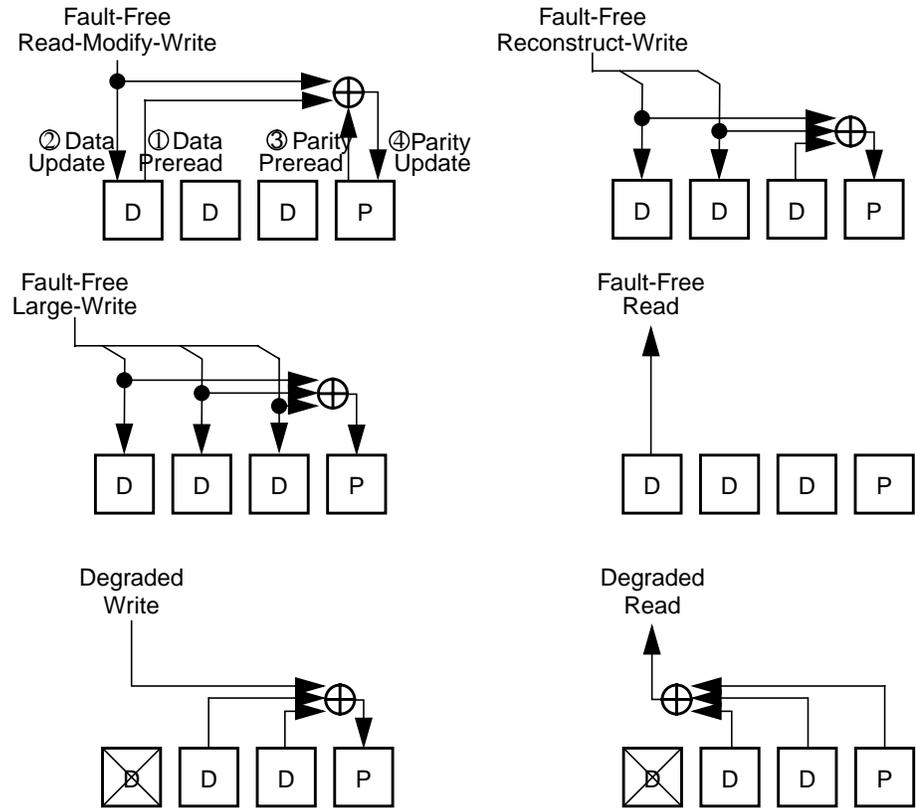
The preread-and-then-write operation performed on the data unit is typically done atomically to minimize the positioning overhead incurred by the access [Stodolsky94]. This is also true for the parity unit. Since the old data must be available to perform the parity update, the data preread-and-write is typically allowed to complete (atomically) before the parity preread-and-write is started.
