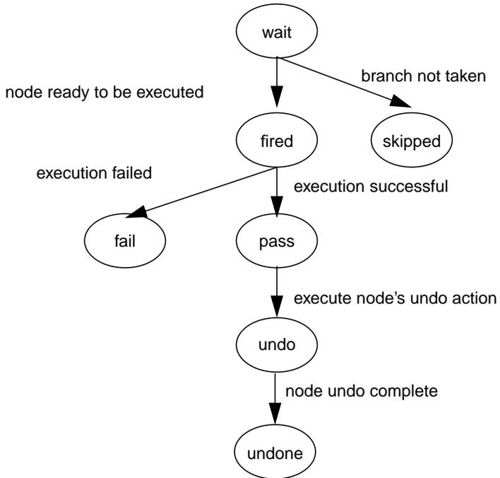
All nodes in a graph begin in the wait state. When a graph successfully completes execution, all nodes are in either the pass or skipped states. The error recovery and undone states, described later in Section 2.5, are reached only if the operation fails.
