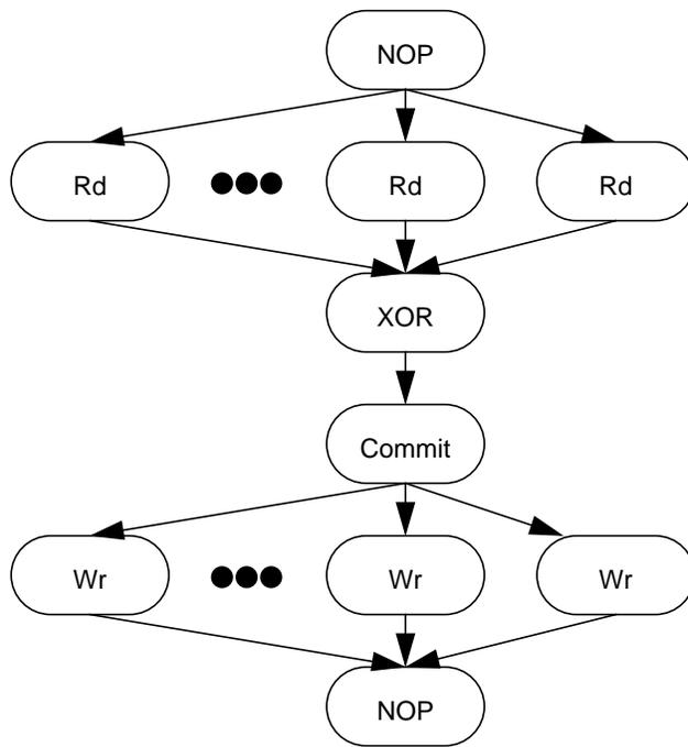
In the reconstruct write operation, illustrated in Figure 23, parity is computed from all symbols in the codeword. The Rd operations collect data symbols which are not being overwritten. Once all data symbols are collected, parity is computed and the new data and parity symbols are written to disk
