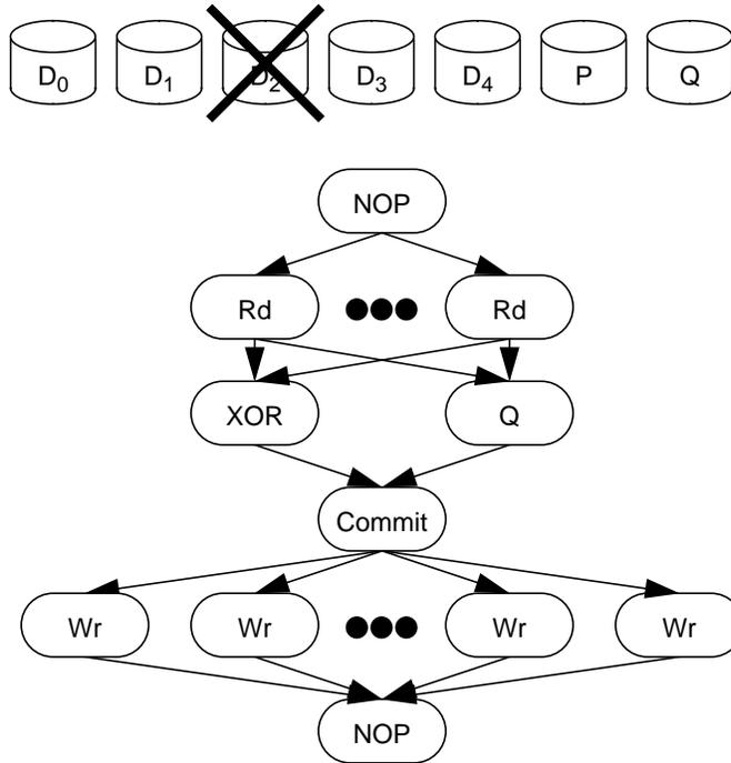
This graph is similar to the reconstruct-write graph (Figure 23) but with an extra chain added to update the “Q” disk. In this example, assume that D<sub>1</sub> and D<sub>2</sub> are to be written. The Rd operations read old data (D<sub>0</sub>, D<sub>3</sub> and D<sub>4</sub>). New values of P and Q are then computed and the writes of D<sub>1</sub>, P, and Q are initiated.. The Commit node blocks all Wr nodes from executing until all new symbols have been computed.
