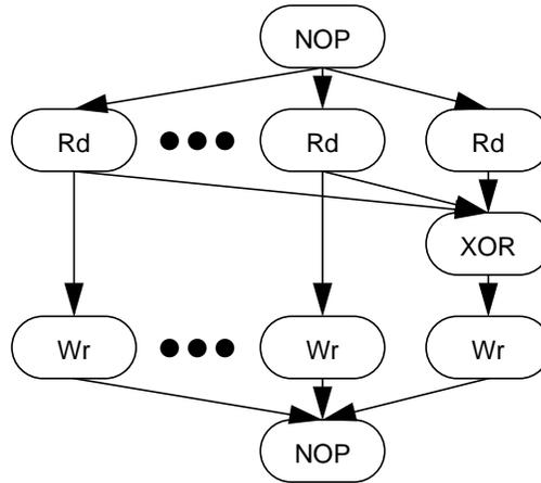
This illustration presents the small write operation. The nodes of the graph are pass-fail actions and the arcs represent the presence of control or data dependencies.
