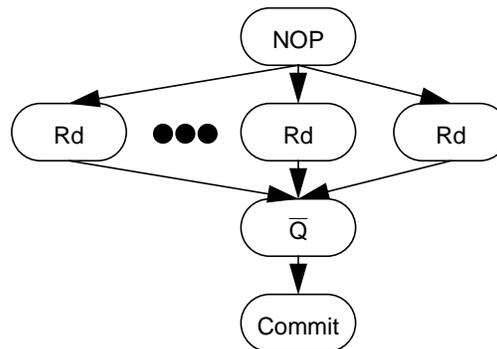
Similar to RAID level 5 arrays, writing less than half of a codeword to a RAID level 6 array is best done using a read-modify-write algorithm. The *PQ small write operation*,
