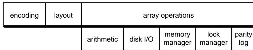
Infrastructure code, which provides the primitive operations from which array operations are implemented, appears in the lower half. Architecture-specific code, such as data encoding, appears in the upper half. When a new architecture is implemented, the infrastructure is unchanged, restricting changes to modules which contain array-specific code.
