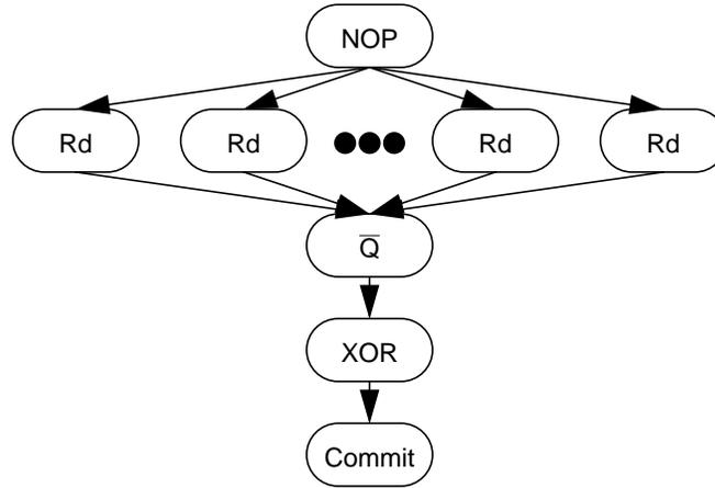
This operation is used when two data units are missing from the codeword. The left-most Rd operation reads the old value of parity and the right-most operation reads the old value of Q. The center Rd operations read all surviving data in the codeword. The Q operation regenerates a single missing data symbol and the XOR node regenerates the other missing symbol.
