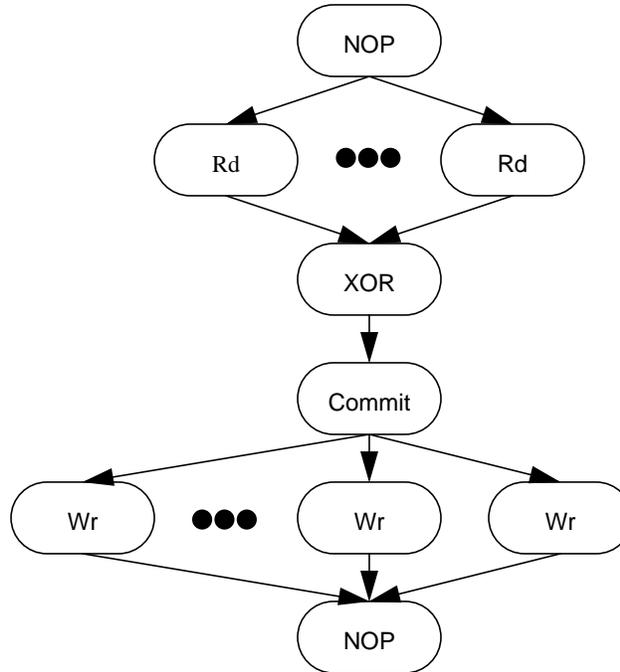
The Rd operations read the data symbols which are not being overwritten. The left-most Wr operations overwrite data symbols and the Wr operation on the right overwrites parity.
