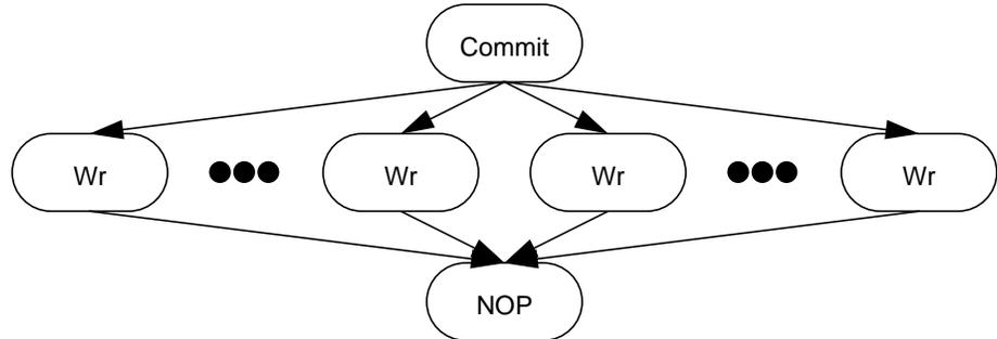
RAID level 1 arrays use copy-based encoding to survive disk faults and require that data must be written to two independent disks. In this graph, the write operations on the left represent writes to a primary disk(s) and write operations on the right represent writes of data to secondary disk(s). The NOP source node of the nonredundant write graph is replaced by a Commit node.
