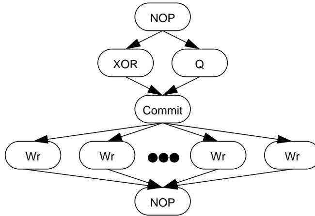
Instead of allowing new data to be written concurrently while the parity overwrite record is computed, the **Commit** node blocks the writes of new data until the **XOR** and **Q** nodes have executed completely.
