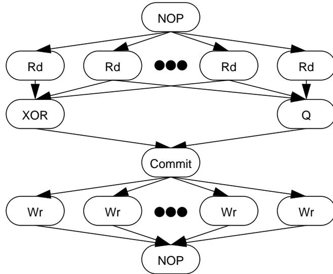
This graph is similar to the small-write graph (Figure 22) but with an extra chain added to update the “Q” disk. The **Commit** node blocks all writes from initiating until all new symbols (data, parity, and Q) have been computed.
