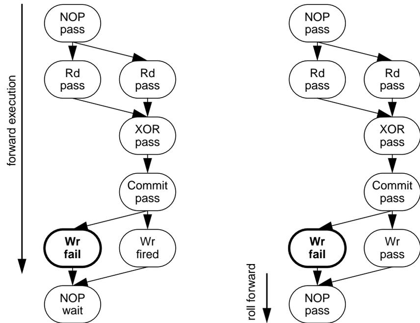
Because the leftmost Wr node failed after the commit point had been reached, forward execution continues. The rightmost Wr node completes successfully as does the sink (NOP) node. If a failure occurs after a commit point, the sink node is always reached and the system appears as if the successful completion of the graph was followed by a failure.
