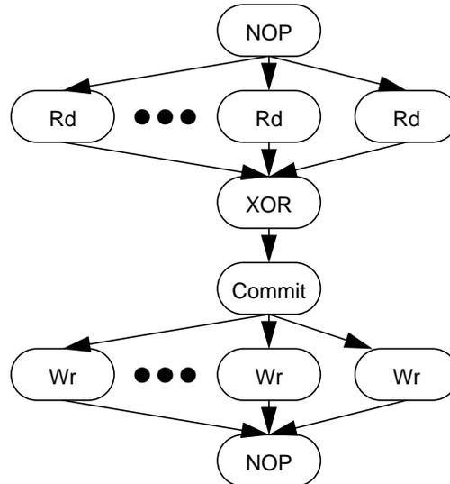
A **Commit** node was inserted to prevent writes of new data from proceeding until all reads of old data and the computation parity have been completed.
