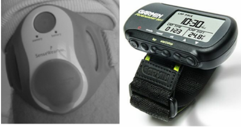
Fig. 2. a) Body sensor fixed on the upper arm. b) Wearable GPS Personal Navigator.
