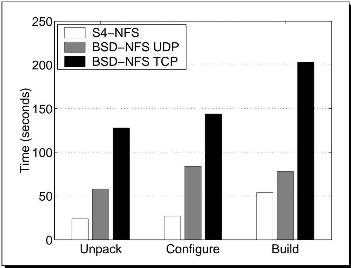
Figure 10: SSH - Unpack, configure, and build.
