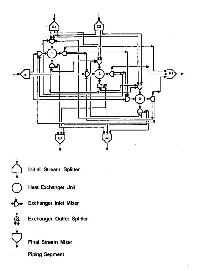
Figure 5 A Three Exchanger Retrofit Superstructure
