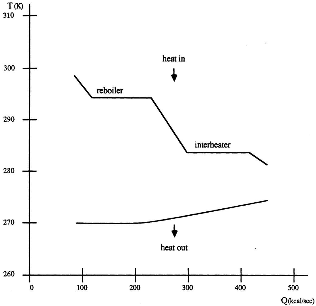
**Figure 8:** Heating (upper) Curve and Cooling (lower) Curve for Example Problem When Feed is Preheated to 50% Vapor. Sloped portions of top curve are heating curve for preheating feed.
