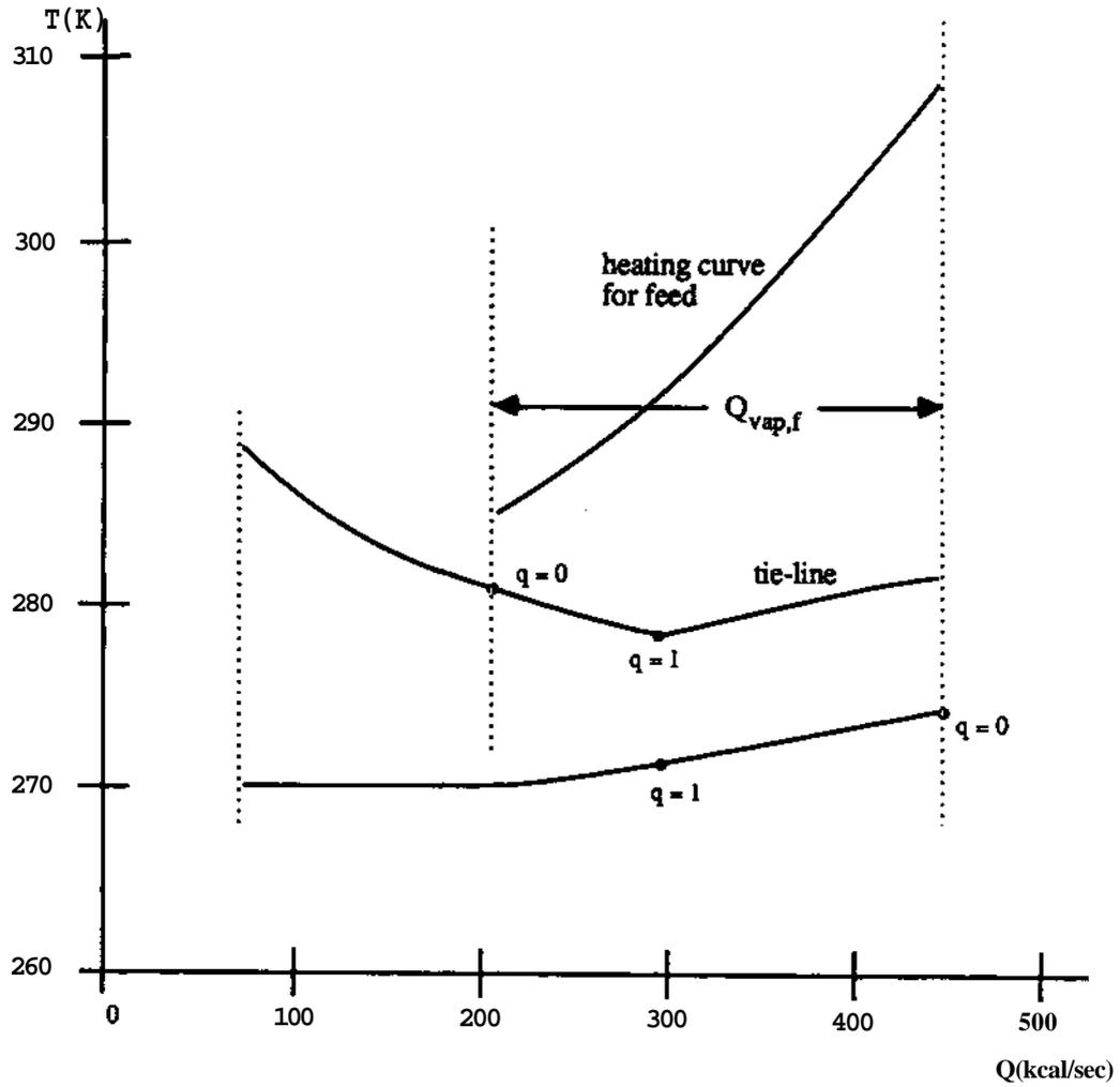
Figure 7: Interheating/Cooling Diagram for Example Problem.
