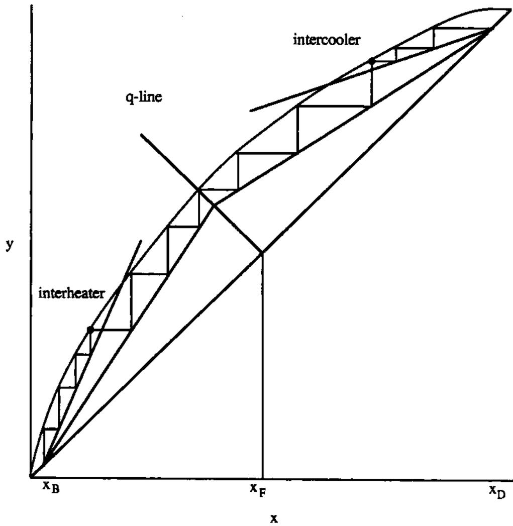
Figure 3: McCabe-Thiele Diagram for Interheated/Intercooled Binary Column
