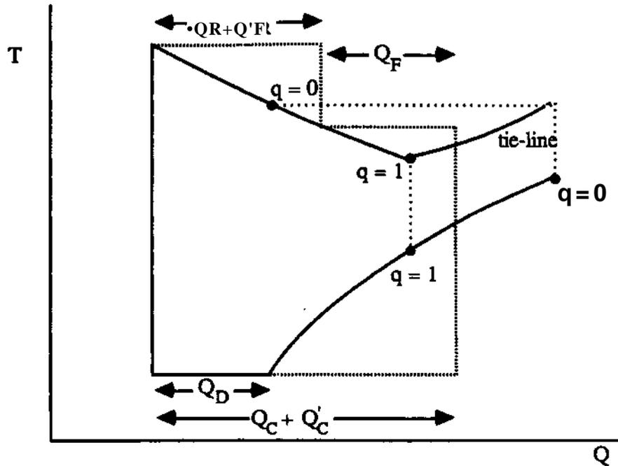
**Figure 6: Interheating/Cooling Diagram for Multicomponent Distillation Column.**
