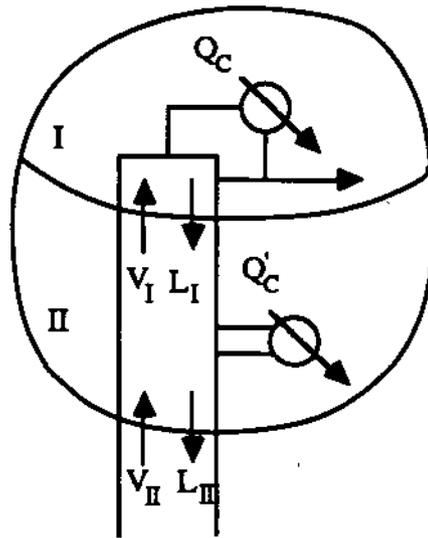
Figure 2: Material and Heat Balance Envelops for Deriving Effect of Intercooling
