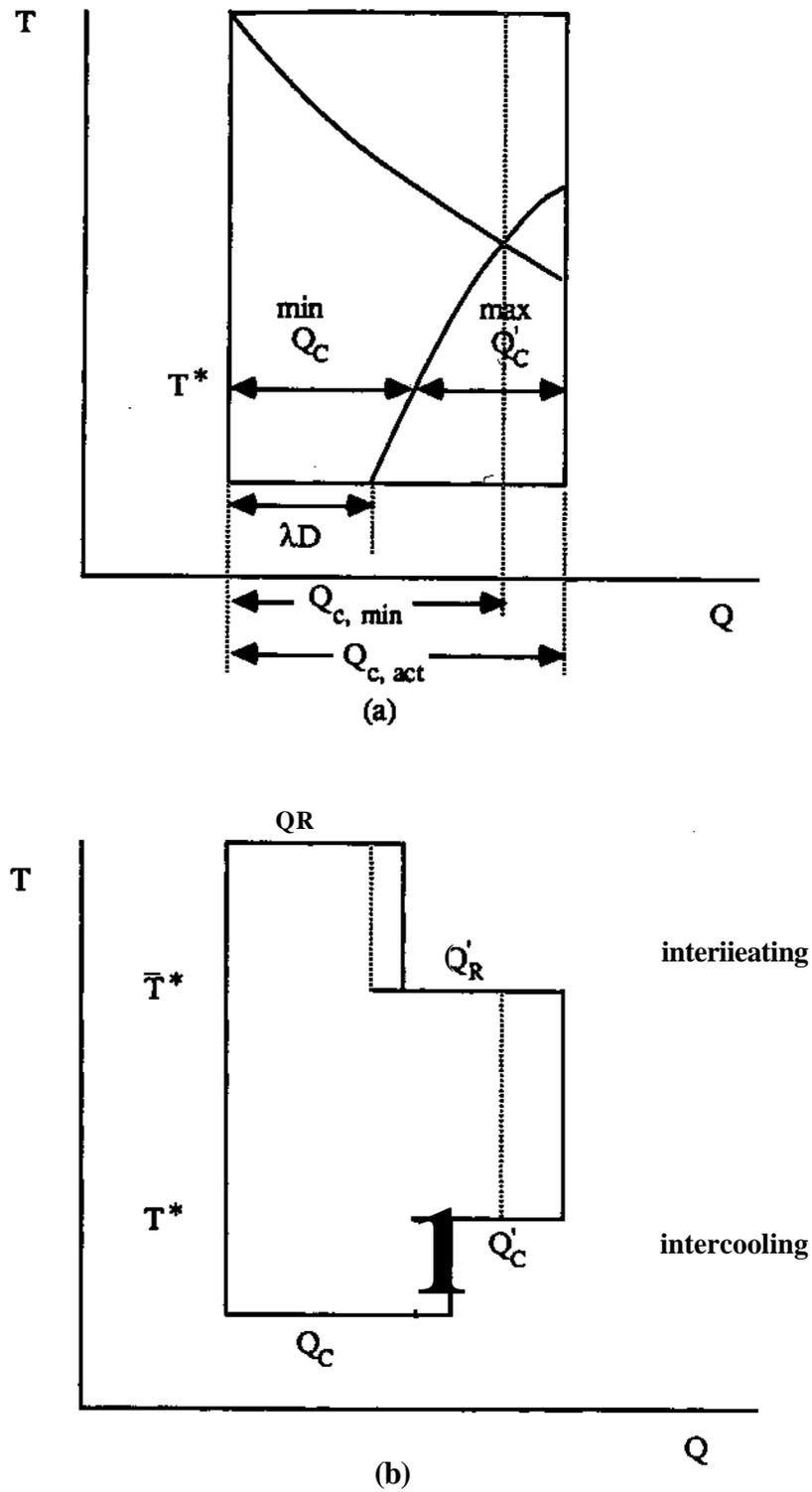
Figure 4: (a) Interheating/Cooling Diagram for Binary Column,
