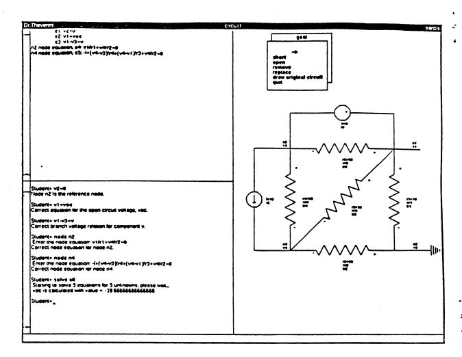
Figure 8: Calculation of voc without any errors
