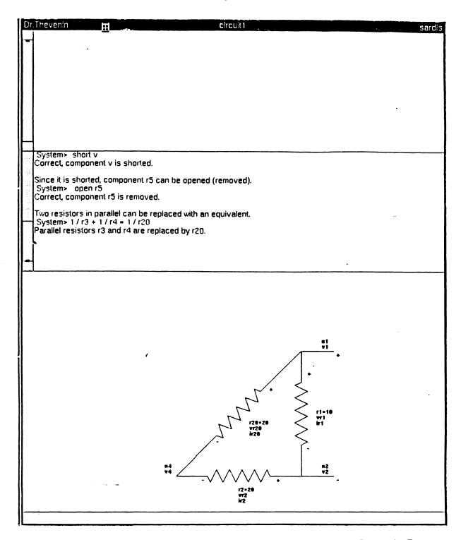
Figure 5: Figure 4 of 6: Illustration of the Problem Solution Method by the System for R<sub>th</sub>
