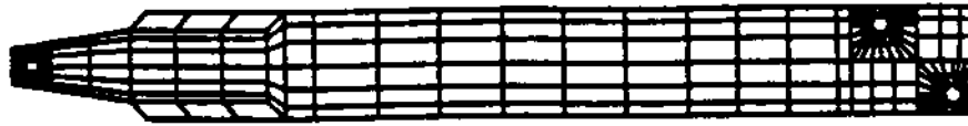
Fig. 7. A finite element mesh for a pen nib. This mesh is generated from the feature diagram (Fig. 3) and provides the input to a commercial finite element analysis program for calculating stresses.
