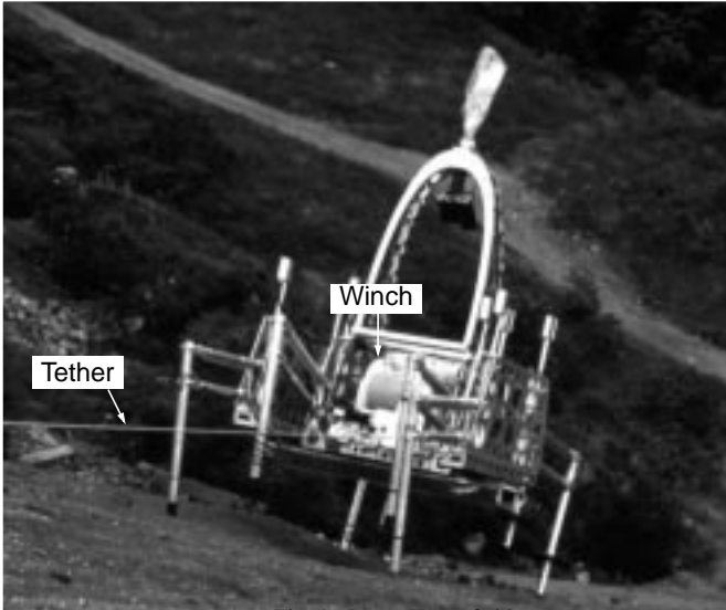
Fig. 1. Dante II at a field test
