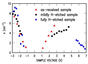
Fig. 6 (color online) Inverse decay length obtained from n-type 6H-SiC samples, as-received and with various amounts of H-etching.
