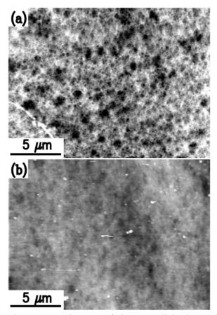
Fig. 1 AFM images of electro-polished 4H-SiC: (a) the  $(000\,\overline{1})$  surface (C-face), and (b) the (0001) surface (Si-face), both displayed with a grayscale range of 33 nm.
