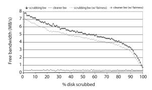
Figure 11: Disk scrubbing and cache cleaning. This figure shows two concurrent background applications, disk scrubbing and cache cleaning, in a system with and without fairness.
