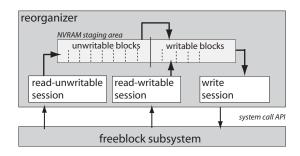
Figure 3: Layout reorganizer architecture. This diagram illustrates the design of the layout reorganizer implemented using our framework. The read-unwritable session manages blocks whose dependencies have not yet been solved. The read-writable session manages all blocks that can be read because their dependencies have been solved. The write session manages all block writes. All data is temporarily stored in the NVRAM staging area.
