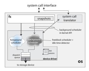
Figure 4: Freeblock subsystem components.
