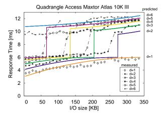
Figure 9: Response time of semi-sequential access.
