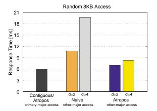
Figure 8: Comparison of response times for random access.
