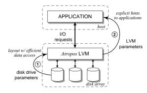
Figure 1: Atropos logical volume manager architecture. Atropos exploits disk characteristics (arrow 1), automatically extracted from disk drives, to construct a new data organization. It exposes high-level parameters that allow applications to directly take advantage of this data organization for efficient access to one- or two-dimensional data structures (arrow 2).
