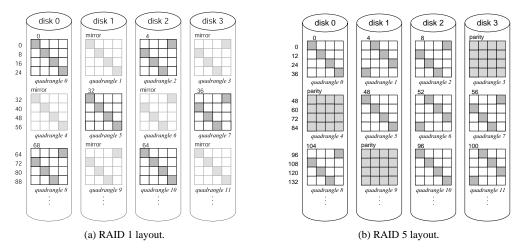
Figure 5: Atropos quadrangle layout for different RAID levels.
