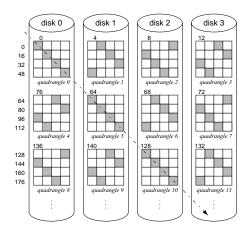
Figure 3: *Atropos* quadrangle layout. The numbers to the left of disk 0 are the *VLBN*s mapped to the gray disk locations connected by the arrow (not the first block of each quadrangle row). The arrow illustrates efficient access in the other-major.
