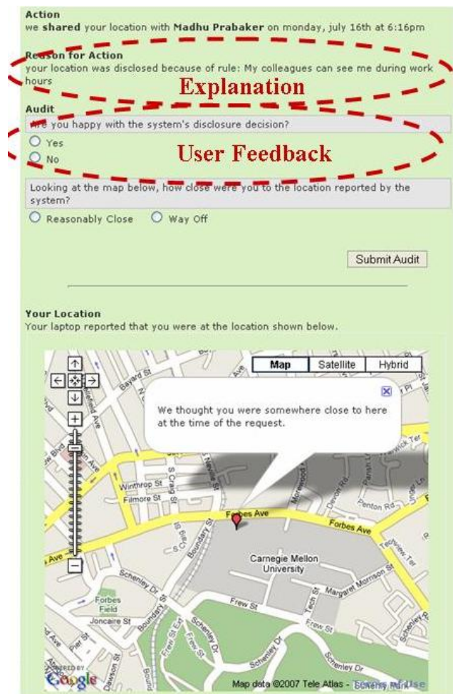
Figure 8. Explanation can help users better understand their policies. User feedback can also be used to make suggestions or learn the user's preferences.
