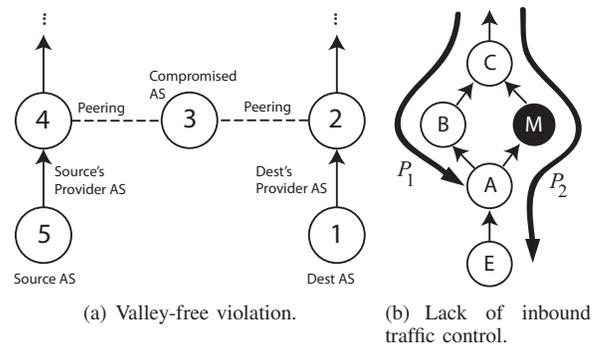
Fig. 1. Arbitrary information flow. Small arrows indicate customer-provider (downstream/upstream) relationships. Large arrows indicate constructed paths. In Figure 1(b),  $P_1$  is preferred by the endpoint  $E$  but  $P_2$  is the path that is used.
