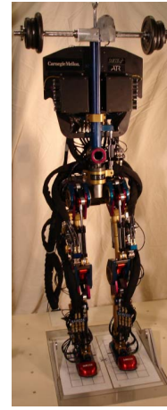
Fig. 4. Sarcos Primus hydraulic biped
