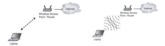
(a) The laptop and the access point figure out precisely where the other is located. The laptop and the access point beam data directly communicate to one another.
