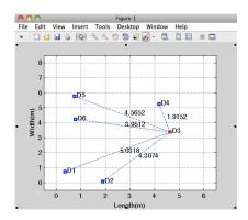
Figure 3: GUI that shows the estimated physical arrangement of devices (represented by blue squares) in the demo.
