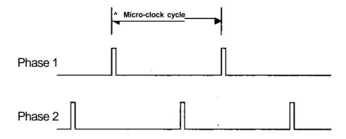
The select signals are valid from the start of a phase 1 cycle to the end of that phase. The evoke signals occur during the phase 2 clock pulse.
