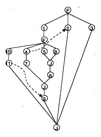
The solid lines indicate the same information which is contained in the forward and backward fields. The dashed lines indicate the the nodes which Cgsame points to. The numbered nodes are the ordinary control graph nodes. The forks and joins are represented by F and J respectively.
